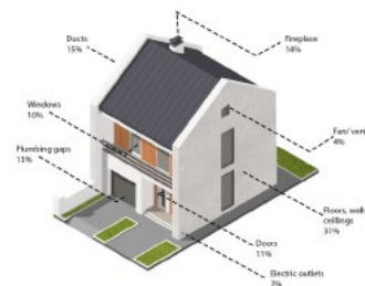
Figure 10: Air leakage in a house
